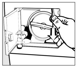
■ Pull the ring of the door mechanism downwards, the door will open.
